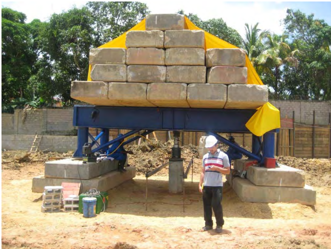
Figure 7.9 - Axial Pile Load test being carried out on a 600 mm CFA Pile (EISL 2010).
