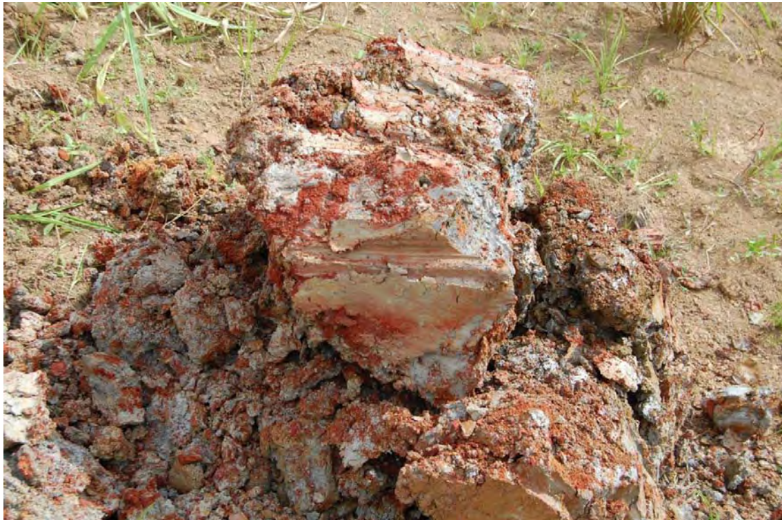
FIGURE. 5.1 - COUVA CHILDREN'S HOSPITAL, COUVA, TRINIDAD – TEST PIT 2 - TOP SOIL OVER MOIST MOTTLED BROWN PLASTIC SILTY CLAYS
