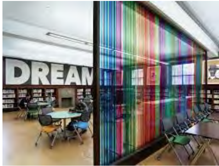
Translucent space dividers to allow natural light transfer through the building
